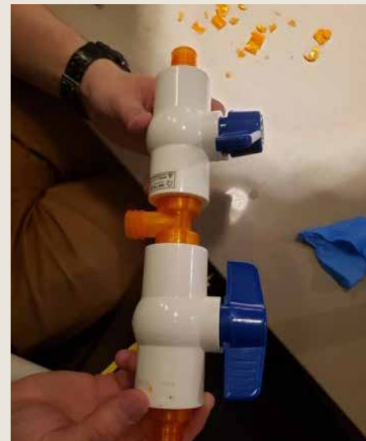
(Left) IDEA Lab designed a two-part air pressure regulator with 3D printed clamps to control air flow to two separate patients using one ventilator. (Right) Students set up makeshift IDEA Lab in their homes to 3D print parts for the ventilator project.
