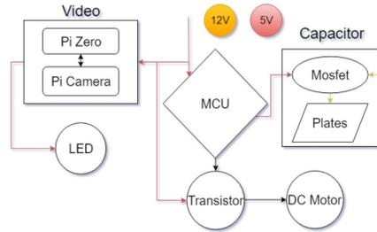
Figure : Functional block diagram for the Small debris Collector
