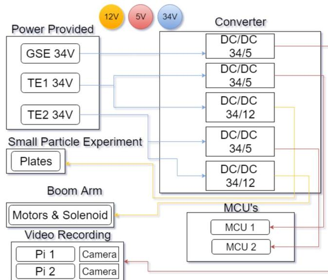
Figure : Functional Block Diagram for Power
