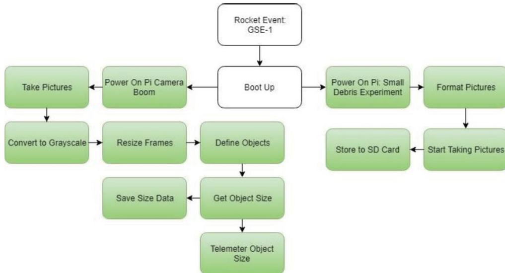
Figure : Software flow chart of Pi cameras.
