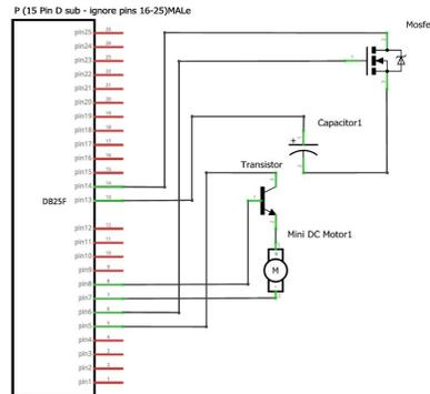
Figure :Wiring diagram for the Small debris Collector
