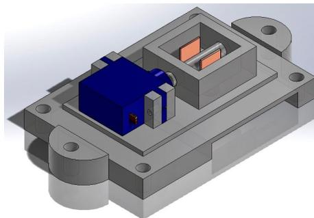
Figure : Base Plate of Small Debris Collector
