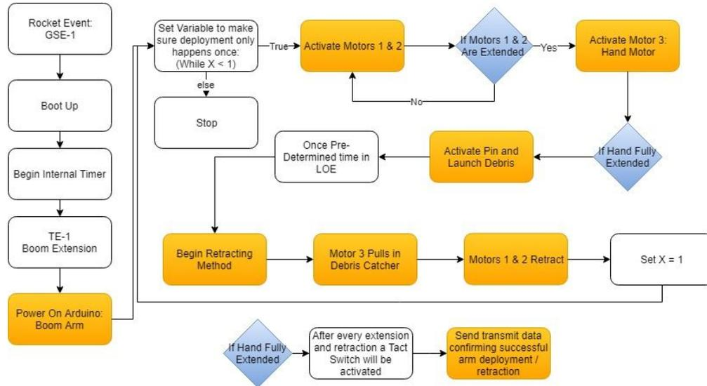
Figure : Software flow chart of main subsystem.
