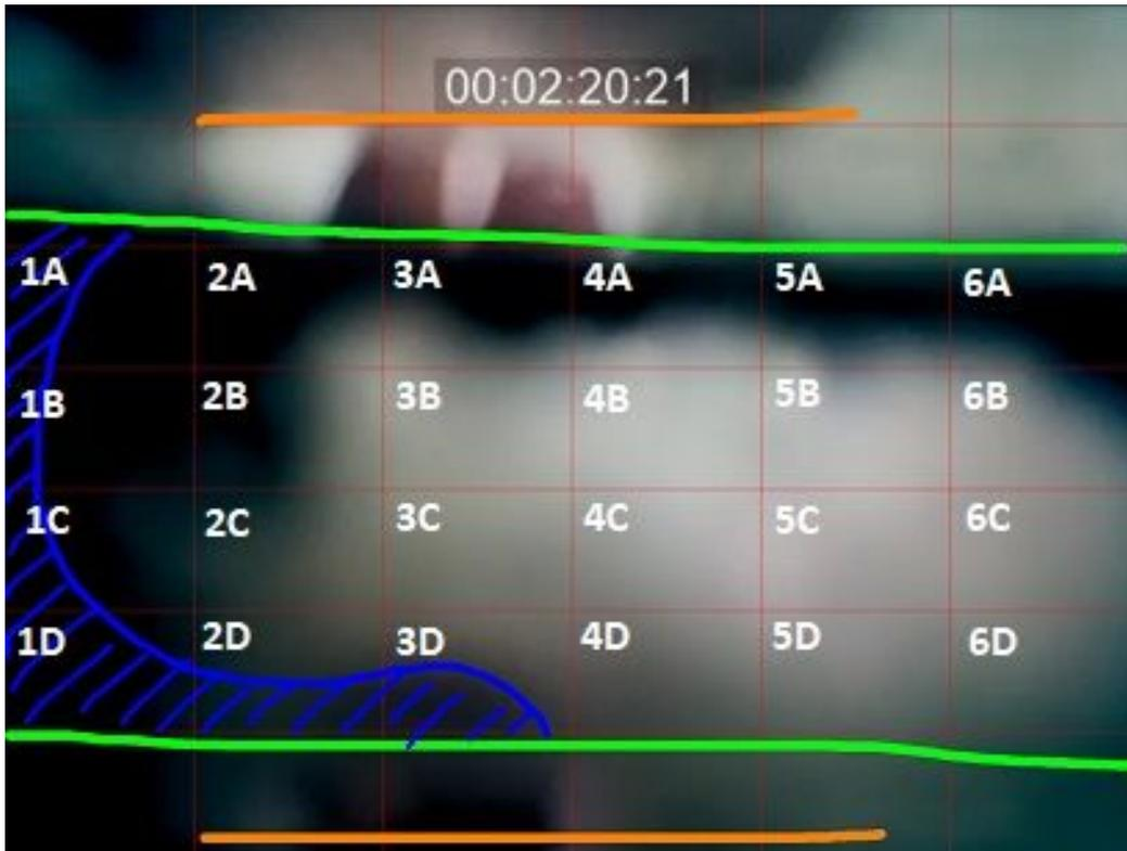
Figure 5: (t = 311 seconds) Beginning of descent. The beads are forced first to the right, toward column 6, and then upward into row A.
