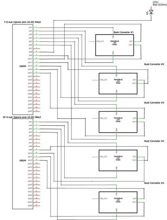
Figure : Electronics diagram for step-down converters
